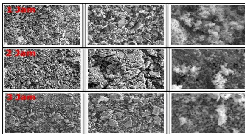
Figure 6. Morphology of hydroxyapatite with sintering duration variation.
