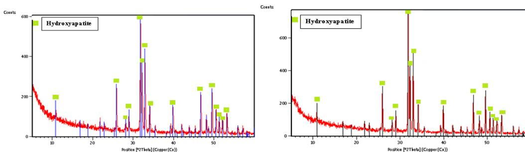
Figure 3. XRD spectrum of Hydroxyapatite at 900°C with duration Variation: (a) 2 hours, (b) 3 hours
