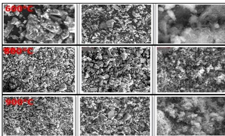
Figure 5. Morphology of hydroxyapatite with sintering temperature variations.
