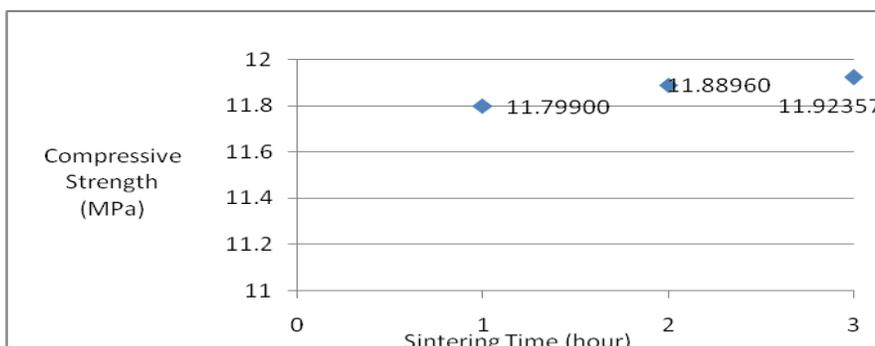
Figure 8: Graph of Hydroxyapatite with Sintering Time Variation
