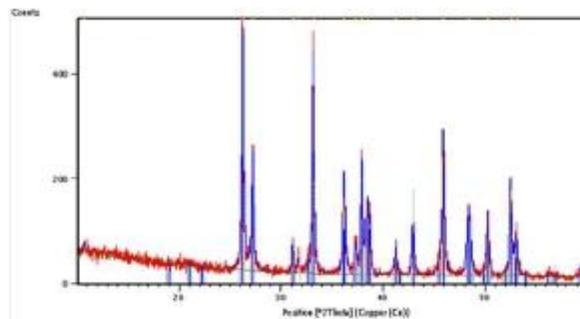
Figure 1: XRD spectrum of cuttlefish bone lamella powders
