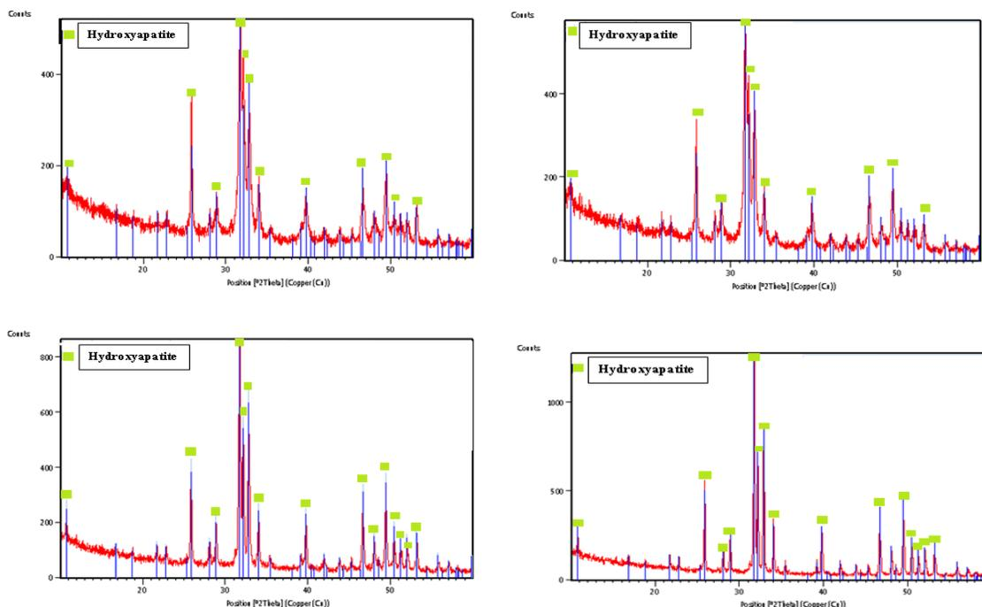
Figure 2. XRD spectrum of Hydroxyapatite with Sintering Temperature Variation (a) Without sinter, (b) 600°C, (c) 800°C, (d) 900°C
