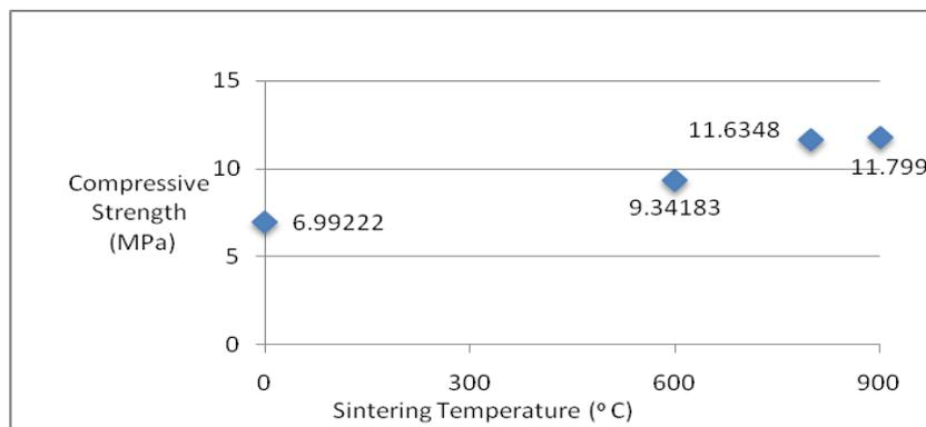
**Figure 7. Graph of Hydroxyapatite with Sintering Temperature Variation**
